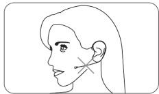
Position the DE50x microphone element about  $0.25^{\circ}-1^{\circ}$  behind the corner of your mouth. Since the DE50x is an omnidirectional capsule, the end of the microphone does not need to be facing your mouth. To avoid breath noise and p-pops, do not place the microphone directly in front of your mouth.
